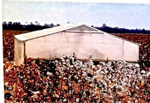
*A rain exclusion tent placed in position in a cotton crop. Air vents are provided at the apex of both ends of the tent to allow flow of moist air from the tent.*
